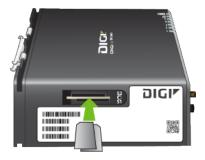
4. After SIM card is installed, use a Philips #1 driver to secure the SIM slot cover. Torque screw to 2 in lbs (225 mN m) maximum.
