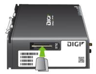
d. After SIM card is installed, use a Philips #1 driver to secure the SIM slot cover. Torque screw to 2 in lbs (225 mN m) maximum.
