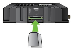
4. After SIM cards are installed, use a Philips #0 driver to secure the SIM slot cover. Torque screw to 2 in lbs (225 mN m) maximum.
