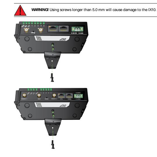
b. Set the IX10 device onto a DIN rail and gently press until the clip snaps into the rail.
